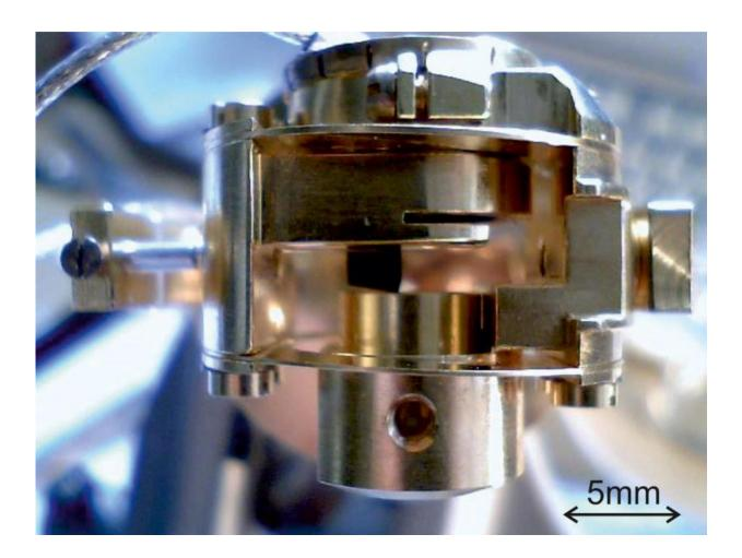
Physicists at Karlsruhe Institute of Technology used this capacitive dilatometer to measure the thermal expansion in cerium copper gold alloys cooled to temperatures very close to absolute zero with a precision of one tenth of a trillionth of a meter, or approximately one-thousandth the radius of single atom. The precise thermal expansion measurements allowed the researchers to map out the stress dependence of entropy in materials as they were cooled to the point of
