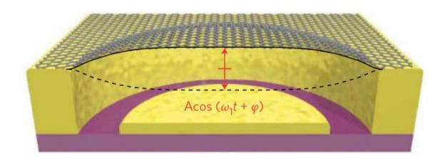
Schematic cross-section of a graphene drum. Credit: ICFO
