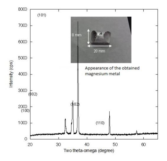
X-ray diffraction result of the obtained magnesium metal. Magnesium peak is observed. Credit: Tokyo Institute of Technology
