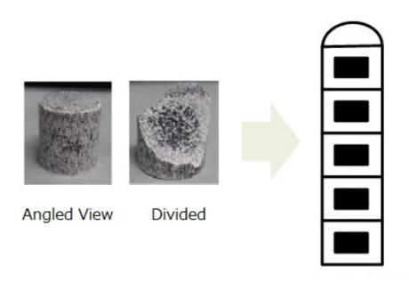
(Left) Actual pellet of dolomite and ferrosilicon. White portion is dolomite rich, and the black portion is ferrosilicon rich. Ferrosilicon is concentrated in the center portion.(Right) Five stacked to form the microwave wavelength (antenna structure). Credit: Tokyo Institute of Technology
