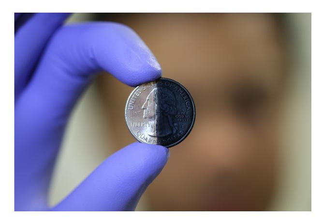
Electroplating can be applied to textured, three-dimensional or flexible substrates, opening the door to new battery designs. The right side of this quarter was plated with lithium cobalt oxide. Credit: Hailong Ning and Jerome Davis III, Xerion Advanced Battery Corp.
