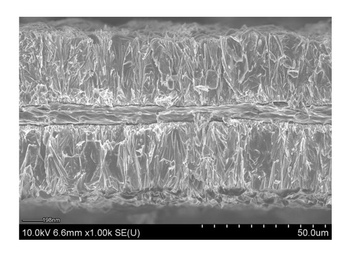
An electron micrograph cross-section shows aluminum foil plated with lithium cobalt oxide, a common material in lithium-ion batteries. Credit: Image courtesy of Hailong Ning and Jerome Davis III, Xerion Advanced Battery Corp.
