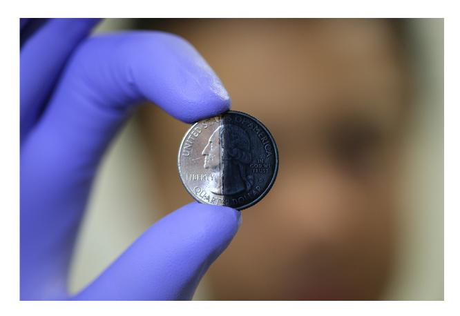
Electroplating can be applied to textured, three-dimensional or flexible substrates, opening the door to new battery designs. The right side of this quarter was plated with lithium cobalt oxide. Credit: Hailong Ning and Jerome Davis III, Xerion Advanced Battery Corp.
