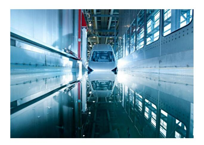
Painting in an immersion bath: Industrial water and paints can be sterilized with electric impulses. Credit: Photo: Eisenmann
