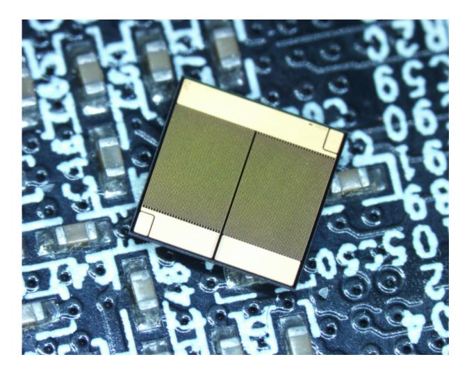
Fraunhofer IAF's monolithically integrated half-bridge circuit. Credit: Photo Fraunhofer IAF
