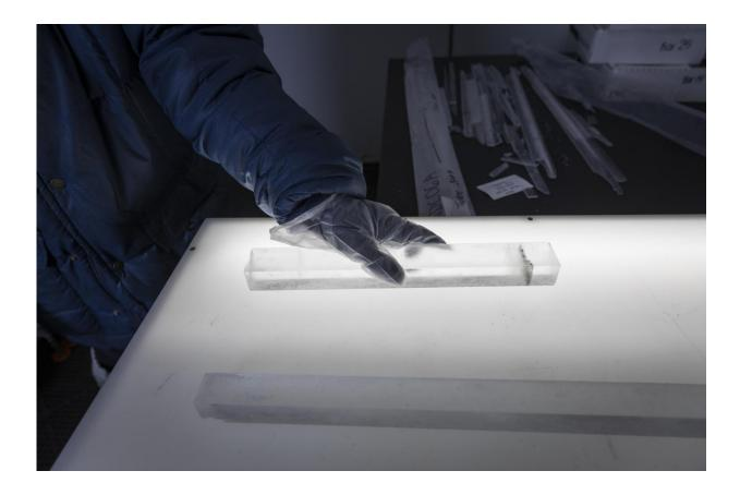
Close-up of an ice core from Antarctica with a darker layer of volcanic ash. The UW group is now analyzing these samples to see if they show the same trend as the Greenland cores. Credit: Mark Stone/University of Washington
