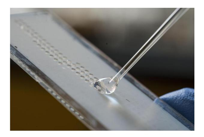
Fluids self-arrange in smallest droplets on a DMA. Credit: KIT
