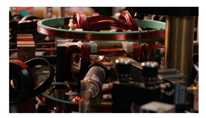
View towards the main experimental chamber of the apparatus, showing the magnetic field coils and optical components required to create the superfluid containing the quantum monopole. See instruction above to access the full-resolution image. Figure 3 caption. Credit: Marcus DeMaio/Amherst College
