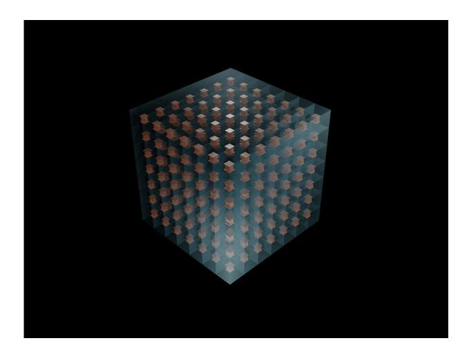
An illustration of how 3-D-printed metamaterial unit cells could be combined like Lego blocks to create structures that bend or focus microwave radiation more powerfully than any material found in nature. Credit: Abel Yangbo Xie, Duke University
