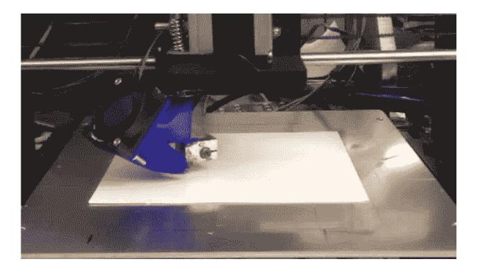
It takes about 20 minutes to 3-D print one metamaterial unit cell using the Electrifi filament and a relatively low-cost 3-D printer. By combining a series of these cells, each tailored to interact with an electromagnetic wave in a certain way, researchers can create a structure that can powerfully manipulate microwave radiation. Credit: Shengrong Ye, Duke University
