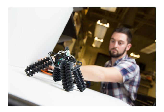
Engineers at the University of California San Diego have developed the first soft robot that is capable of walking on rough surfaces, such as sand and pebbles. The 3-D-printed, four-legged robot can climb over obstacles and walk on different terrains. Credit: Jacobs School of Engineering/UC San Diego
