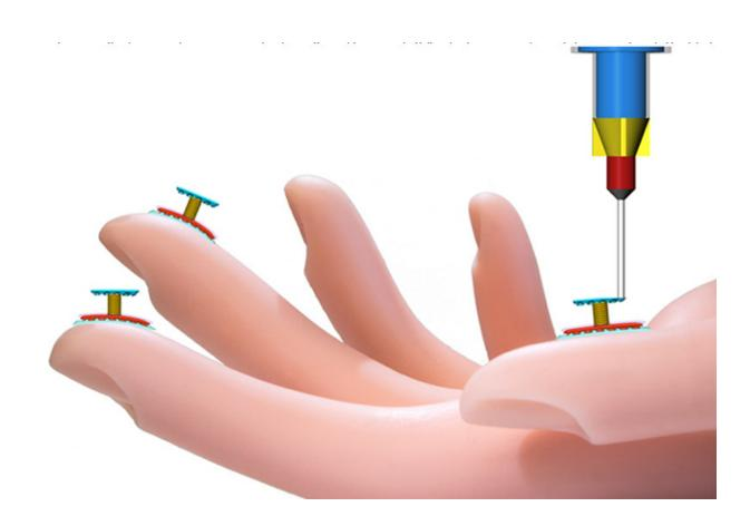
A one-of-a-kind 3D printer built at the University of Minnesota can print touch sensors directly on a model hand. Credit: Shuang-Zhuang Guo and Michael McAlpine, University of Minnesota, "3D Printed Stretchable Tactile Sensors," Advanced Materials. 2017. Copyright Wiley-VCH Verlag GmbH & Co. KGaA.
