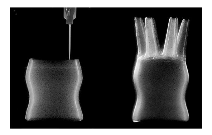
Liquid silicone is 3-D printed into a micro-organogel support to create a perfusable tube network. Once cured and removed from the support material, water is pumped through the printed structure. Credit: O'Bryan et al. Sci. Adv. 2017;3:e1602800
