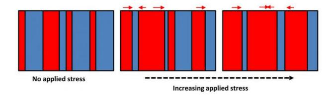
Illustration shows that in response to an applied stress, such as bending, the boundaries of the ferroelastic domains (red and blue regions depict domains oriented in different directions) become bigger or smaller. Credit: NIST
