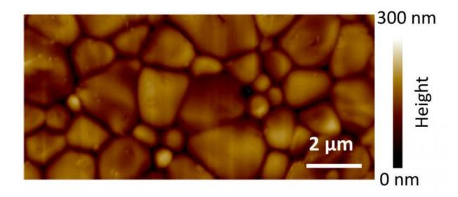
Image recorded by an atomic force microscope reveals the topography of a polycrystalline sample of the perovskite, including the boundaries between crystals. Credit: NIST
