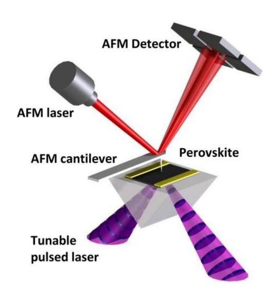
Schematic shows a perovskite sample (black) examined by the photothermal induced resonance technique. When the sample absorbs pulses of light (depicted as disks in purple cones), the sample expands rapidly, causing the cantilever of
