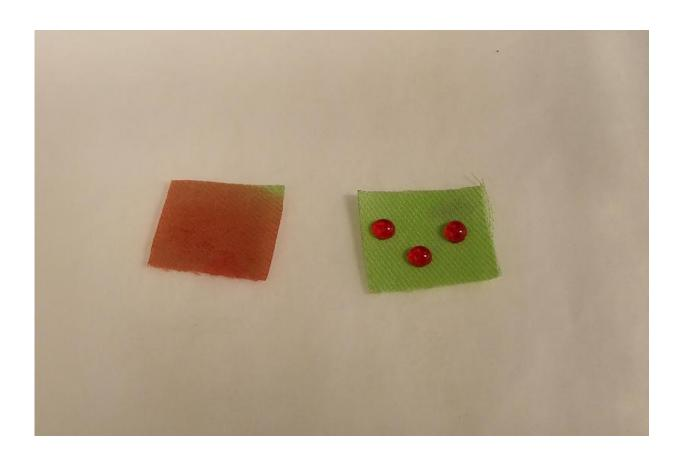
Samples of cloth both untreated, left, and treated with a fluorine-free oleophobic coating developed in the labs of Emmanuel Giannelis, professor of materials science and engineering, and Jintu Fan, professor of fiber science & apparel design. The oil beads up and can be easily removed from the treated material. Credit: Genggeng Qi/Provided
