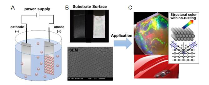
A) Illustration of the electrophoretic deposition (EPD) of sulfone-containing nano-latex shows negatively charged nano-particles in suspension migrating towards the positive electrode. B) The anode coated with aligned nano-particles (top: electrode, bottom: SEM image. Scale bar, 2000 nm). C) Images of application example and the light reflection by the colorless nano-particles. Credit: NITECH
