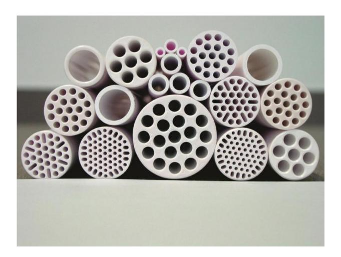
Ceramic membranes by the Fraunhofer Institute for Ceramic Technologies and Systems IKTS. Credit: Fraunhofer IKTS
