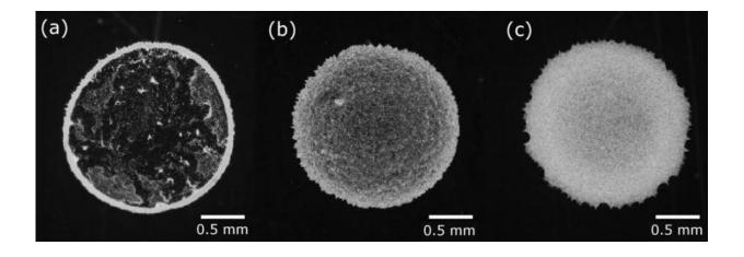
Photographs of dried colloidal mixtures of polystyrene particles (diameter 1.4  $\mu$ m) and cellulose fibers (diameter ca. 20 nm, length ca. 1  $\mu$ m). The polystyrene concentration is fixed at 0.1 wt%, and that of cellulose is 0 (a), 0.01 (b) and 0.1 wt% (c). Credit: National Institute for Materials Science
