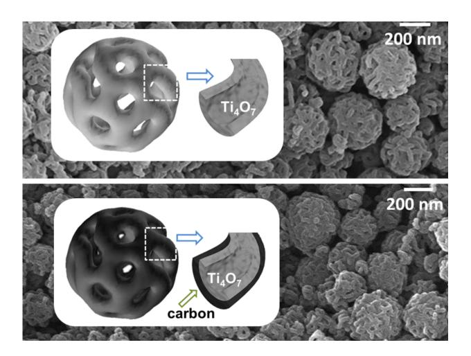
The porous structure of the nanoparticles is visible under the electron microscope. Credit: HZB/adfm.201701176
