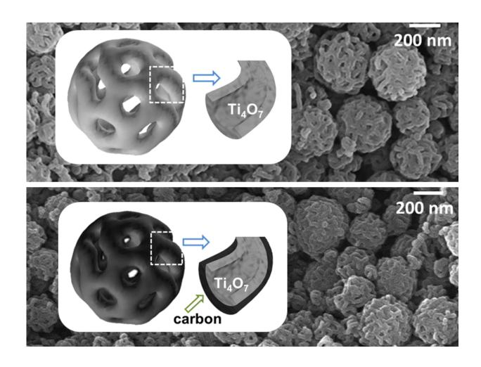
The porous structure of the nanoparticles is visible under the electron microscope. Credit: HZB/adfm.201701176
