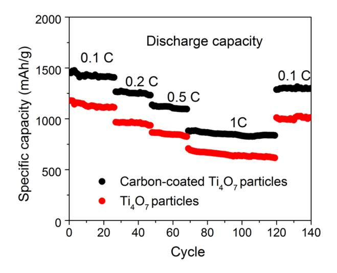
The specific capacity declines very little during repeated charge/discharge cycles. Credit: HZB/adfm.201701176
