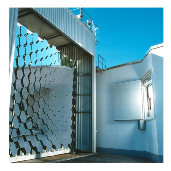
The solar furnace at the DLR German Aerospace Center facility in Cologne has two working setups. As a baseline, 147 curved mirrors focus sunlight into a high-temperature beam. But the weather in northern Europe does not always cooperate, so the sun is sometimes simulated by an array of xenon lamps more typically found in cinema projectors. Credit: DLR
