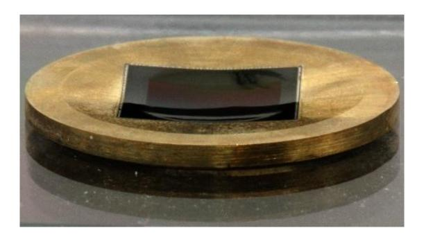
Researchers developed a way to create spherically curved image sensors by threedimensionally bending off-the-shelf image sensors. When incorporated into prototype cameras, the curved sensors produced greatly improved image quality compared to high-end commercial cameras. Credit: Microsoft Research
