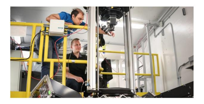
Researchers Abhijit Pramanick of the City University of Hong Kong (left) and Mads Ry Jørgensen of Aarhus University are studying ferroelectric properties on TOPAZ, SNS beam line 12, to better understand how ferroelectric materials behave under high temperatures and the application of electric fields. Their research could also lead to the development of more environmentally friendly materials. Credit: ORNL/Genevieve Martin
