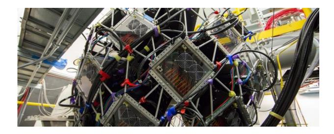
TOPAZ is an elastic scattering instrument that allows for probing of material structures and responses under controlled environmental conditions. It enables neutron measurement of the same single-crystal samples that is possible with x-ray diffraction. Credit: US Department of Energy
