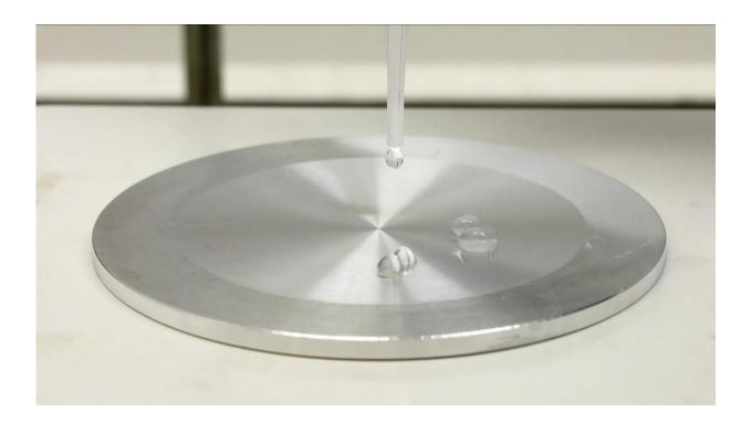
Leidenfrost effect makes water droplets on a hot plate hover over the surface instead of making physical contact with it. Credit: Aalto University / Mikko Raskinen
