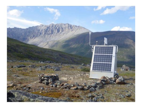
This undated photo provided by Incorporated Research Institutions for Seismology shows a seismic station installed at Anaktuvak Pass in Alaska's Brooks Range. The station sends out earthquake information in real time. A seismometer rests at the bottom of a borehole and a fiberglass hut equipped with solar panels protects the station power system, electronics and radio telemetry equipment. (Incorporated Research Institutions for Seismology via AP)
