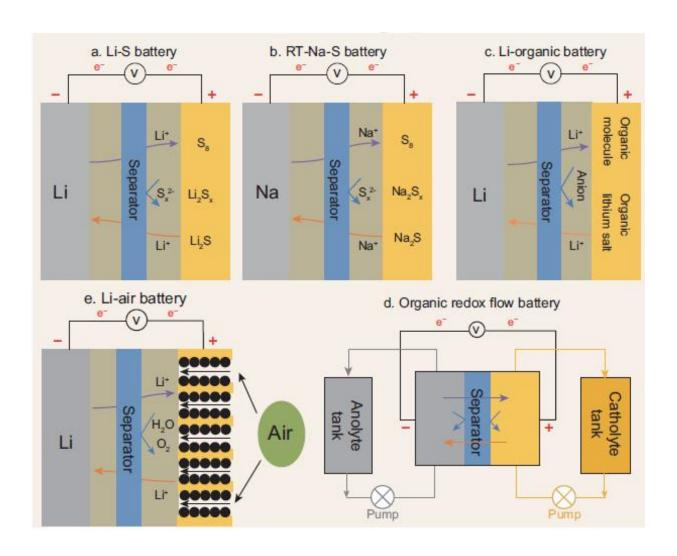
(a) Li-S, (b) room-temperature Na-S, (c) Li-organic, (d) organic-based redox-flow, and (e) Li-air batteries. Credit: ©Science China Press
