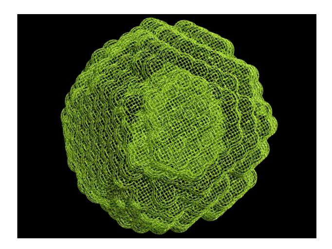
This image illustrates that, as iron oxide undergoes oxidation, voids in the nanoparticles merge to form crescents. Credit: Alexandra Kirby / Y. Sun et al. / *Science* (2017)
