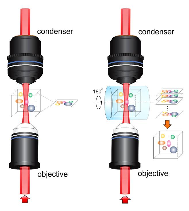
This schematic depicts an imaging system that uses a special type of laser beam called a Bessel beam that is produced using a pair of cone-shaped "axicon" lenses combined with a microscope objective. Purdue University researchers are using the system, which is able to penetrate deep into tissue and might lead to technologies that eliminate the need to draw blood for analyses including drug testing and early detection of diseases such as cancer and diabetes. Credit:
