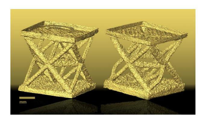
In situ compression results for a 10 percent octet structure show the force versus displacement plot for the same octet sample. At left, the 3D tomography surface under no load and at right, after the onset of an elastic deformation.
