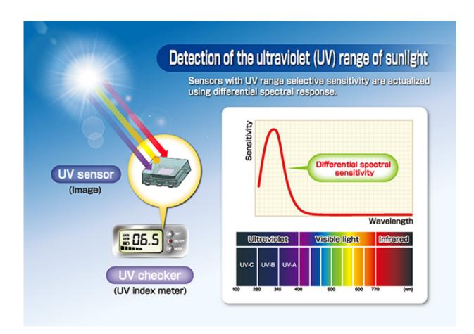
The new UV light sensor technology uses only silicon semiconductors to selectively detect and measure the light intensity of UV-A and UV-B light wavebands. Credit: Tohoku University
