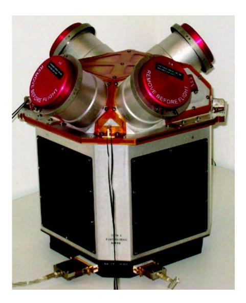
This cluster of four colloid thrusters is part of the Disturbance Reduction System, developed by NASA/JPL, which will help keep the LISA Pathfinder spacecraft extremely stable. Credit: ESA/NASA/JPLCaltech
