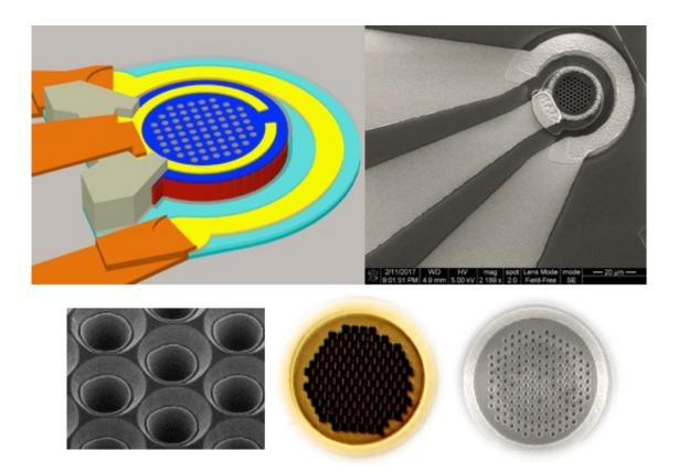
Photodetectors for optical to electronic signal conversion usually make use of efficient, but expensive materials other than silicon. A new approach uses tapered holes in silicon to trap photons and send them sideways through a silicon wafer, boosting efficiency. The approach allows high-efficiency, high-speed photodetectors that could be cheaper and more efficient for use in data centers. Credit: Saif Islam, UC Davis
