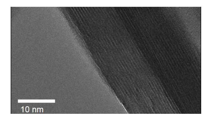
Low temperature high resolution transmission electron microscope image of a platelet of tungsten oxide dihydrate; the "stripes" are individual layers of atoms separated by water layers. Credit: North Carolina State University
