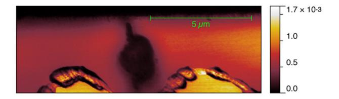
The rough, bright patches reveal details of the never-before-seen damage dealt by the helium ion beam used to carve channels in an attempt to create the conditions for superconductivity. Credit: Brookhaven National Laboratory
