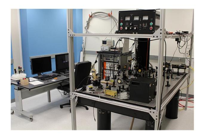
The new instrument, developed at Brookhaven and in use at Yale, combines atomic force microscopy (AFM) and scanning near-field optical microscopy to provide unprecedented insight into these complex nanomaterials. Credit: Adrian Gozar
