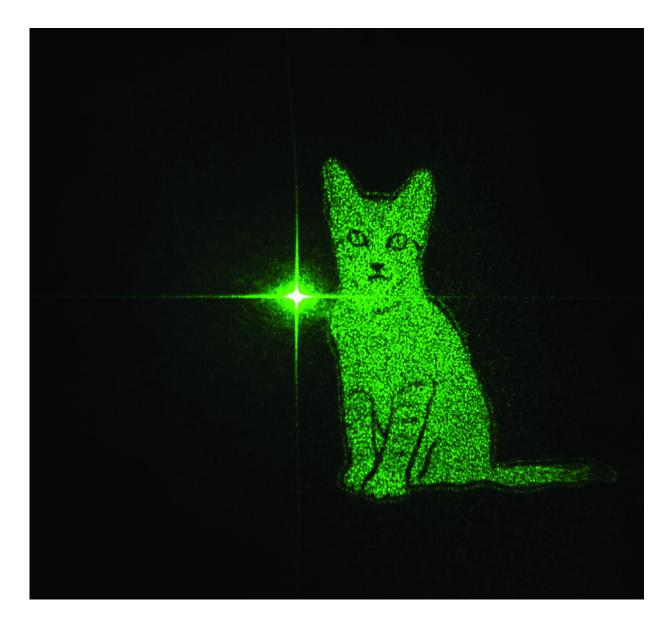
This hologram is one of two different holographic images encoded in a metasurface that can be unlocked separately with differently polarized light Credit: The Capasso Lab/Harvard SEAS
