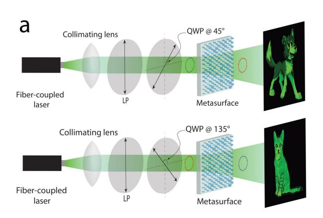
A single metasurface encodes two separate holograms. When illuminated with one direction of polarized light, the metasurface projects an image of a cartoon dog. When illuminated with the perpendicular direction of light, the metasurface projects an image of a cartoon cat. Credit: The Capasso Lab/Harvard SEAS
