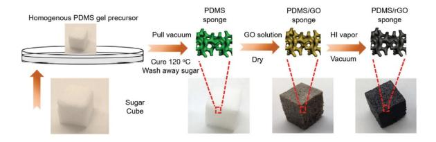
A sugar cube serves as a template for new stretchable, sponge-like, graphenebased battery electrodes. Credit: Li et al. ©2017 WILEY-VCH
