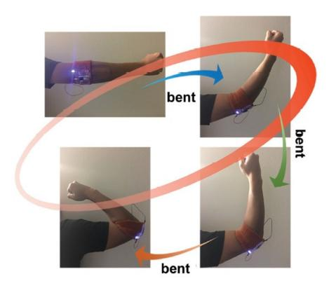
The stretchable sodium-ion full battery is attached to an athletic elbow brace under different bending states, where it continuously powers a commercial LED light. Credit: Li et al. ©2017 WILEY-VCH
