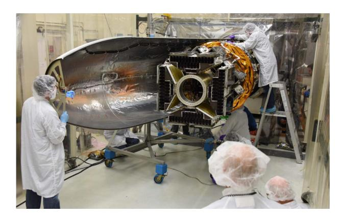
These SwRI-designed and -built spacecraft, eight microsatellites for NASA's Cyclone Global Navigation Satellite System (CYGNSS) mission (shown during payload integration), recently transitioned into operations phase after a December 2016 launch into low-Earth orbit. The CYGNSS mission is designed to measure the ocean surface beneath a hurricane to allow scientists to predict wind speed and how strong a storm will be when it makes landfall. Credit: Southwest Research Institute
