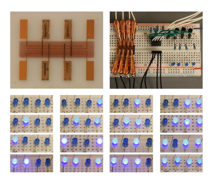
Duke University researchers have developed a new 'spray-on' digital memory (upper left) that could be used to build programmable electronic devices on flexible materials like paper, plastic or fabric. To demonstrate a simple application of their device, they used their memory to program different patterns
