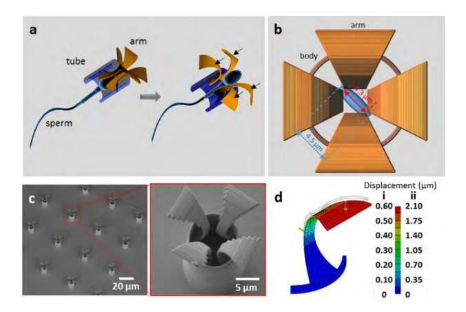
(a) Schematic illustration of the sperm-hybrid micromotor and the sperm release process. Black arrows represent the reactive force on the arms upon hitting an obstacle.(b) Top view of the tetrapod microstructure with schematic sperm head(c) SEM images of an array of printed tetrapod microstructures.(d) Simulation results demonstrating the deformation of one single arm. Yellow arrows represent the applied forces.(i) Applied force is 128 pN from a motile, non-
