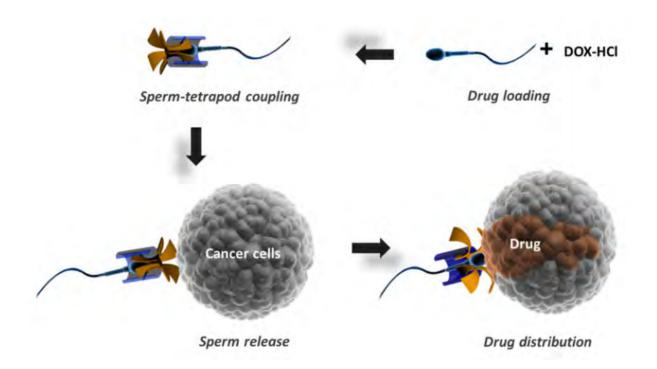
Schematic depicting tumor targeted drug delivery by a sperm-hybrid micromotor under magnetic guidance with mechanical sperm release trigger. Credit:
