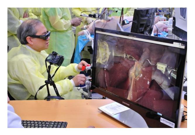
The robotic arms are highly sensitive to touch, have up to ten degrees of movement, and can perform surgical procedures by means of a single incision. Credit: The Hong Kong Polytechnic University
