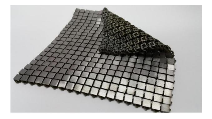
Another example of a 3-D-printed metallic "space fabric." The bottom and top sides of the fabric are designed to have different functionality. Credit: NASA/JPL-Caltech
