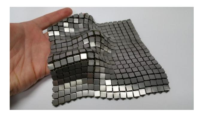
This metallic "space fabric" was created using 3-D printed techniques that add different functionality to each side of the material. Credit: NASA/JPL-Caltech
