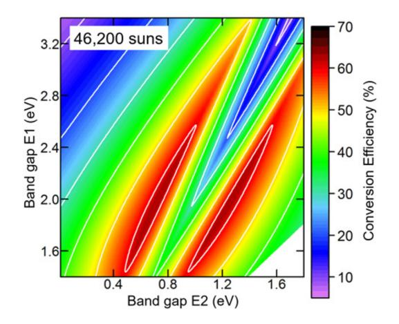
Theoretical prediction of conversion efficiency. The efficiency changes in response to the use of two different bandgaps in a hetero-interface. The highest conversion efficiency is 63%. Credit: Kobe University
