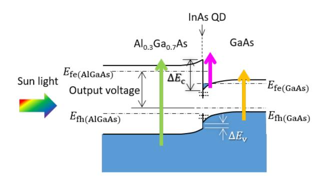
A solar cell structure using a hetero interface and the up-conversion of the twoproton system (yellow and red arrows). The light represented by the red and yellow arrows normally passes through when only a semiconductor is used, but with this system the light is absorbed, greatly increasingly the flow of electricity. Credit: Kobe University
