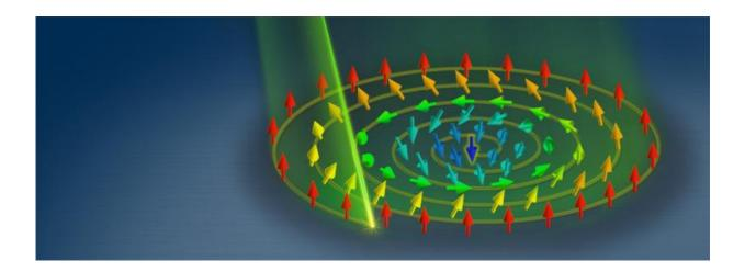
Argonne researchers have created skyrmions – ordered regions of magnetic spins – by using a spiraling focused ion beam. Credit: Robert Horn / Argonne National Laboratory
