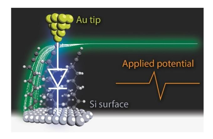
Single-molecule diode formed by sandwiching a molecule between a gold and a silicon electrode. Credit: I Díez-Pérez
