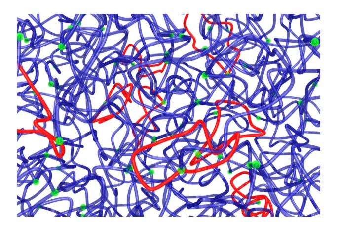
Researchers have found a new approach for reducing the number of loops (red) in a polymer. The method could offer an easy way for manufacturers of industrially useful materials such as plastics or gels to strengthen their materials. Credit: Massachusetts Institute of Technology
