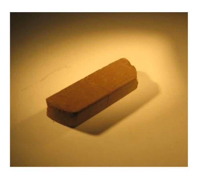
A brick made of Martian soil simulant compacted under pressure. The brick was made without any additional ingredients and without baking. Credit: Jacobs School of Engineering/UC San Diego
