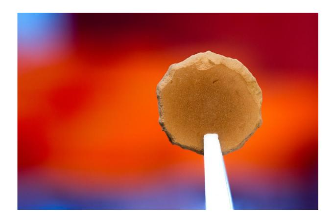
Researchers compacted Mars simulant under pressure in a cylindrical, flexible rubber tube. This is what the result of the experiment looked like before it was cut into bricks. Credit: Jacobs School of Engineering/UC San Diego
