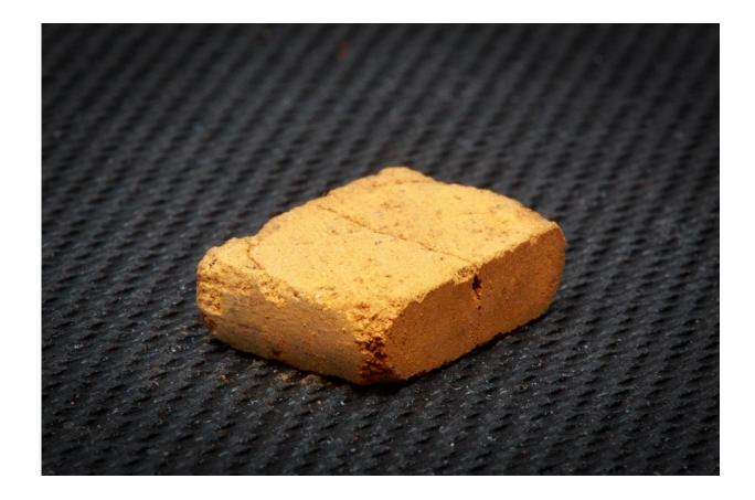
Researchers investigated the bricks' strengths and found that even without rebar, they are stronger than steel-reinforced concrete. Here is a sample after testing to the point of failure. Credit: Jacobs School of Engineering/UC San Diego
