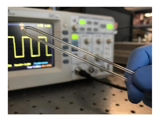
A glass tube sensor developed by engineers at the University of California, Riverside will allow scientists to weigh tiny biological samples in their native liquid environments. Credit: UC Riverside
