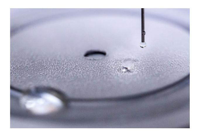
A water droplet bounces off a hydrophobic coating on a surface that has been burned and abraded in the NCRC on March 28, 2017. Credit: Joseph Xu/Multimedia Content Producer, University of Michigan - College of Engineering
