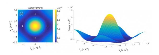
Plot of polaritons' energy dispersion vs momentum in a semiconductor microcavity, seen from above (left) and the side (right). Minimal energy locations, called valleys, are shown with white crosses. Credit: Institute for Basic Science
