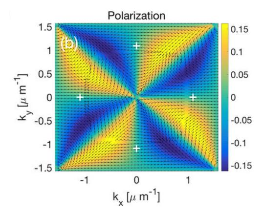
Model of valleys with different polarizations. The model uses vectors (arrows) and colors (from yellow to blue) to show opposite polarizations on different valleys (white crosses). The opposite polarizations (arrow direction) can be, in principle, excited selectively by a polarized laser. Credit: Institute for Basic Science
