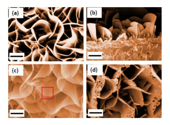
a) Colorized SEM images of iron oxide nanoblades used in the experiment. b) Colorized cross-section of SEM image of the nanoblades. c) Colorized SEM image of nanoblades after 1 hour of reduction reaction at 500 °C in molecular hydrogen, showing the sawtooth shape along the edges (square). d) Colorized SEM image showing the formation of holes after 2 hours of reduction. The scale bar is 1 micrometer. Credit: W. Zhu et al./ACS Nano and K. Irvine/NIST
