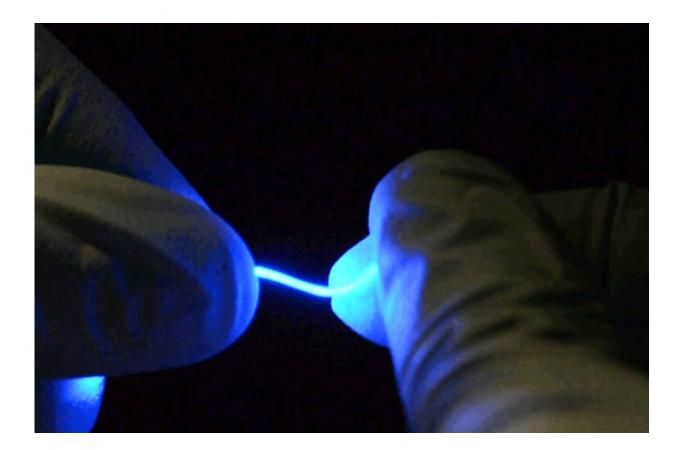
Researchers have developed a rubber-like fiber, shown here, that can flex and stretch while simultaneously delivering both optical impulses, for optoelectronic stimulation, and electrical connections, for stimulation and monitoring. The fibers are not only stretchable but also very flexible. "They're so floppy, you could use them to do sutures, and do light delivery at the same time," professor Polina Anikeeva says. Credit: Chi (Alice) Lu and Seongjun Park
